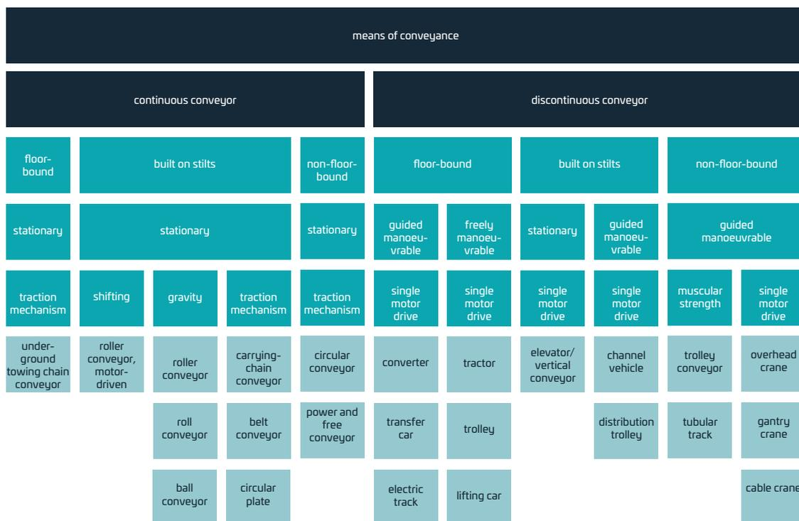
Figure 3 Classification of conveyor for transporting package goods according to Hompel (Hompel 2018 p.129)
